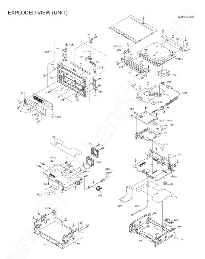
Parts with the exploded numbers lager than 700 are not supplied.
