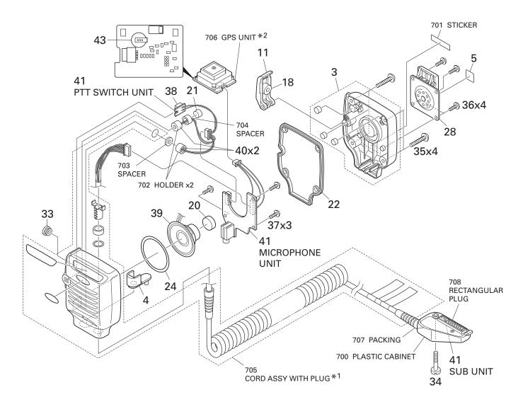
\*1: In order to maintain the waterproofing performance, the cord ASSY with plug cannot be replaced.
