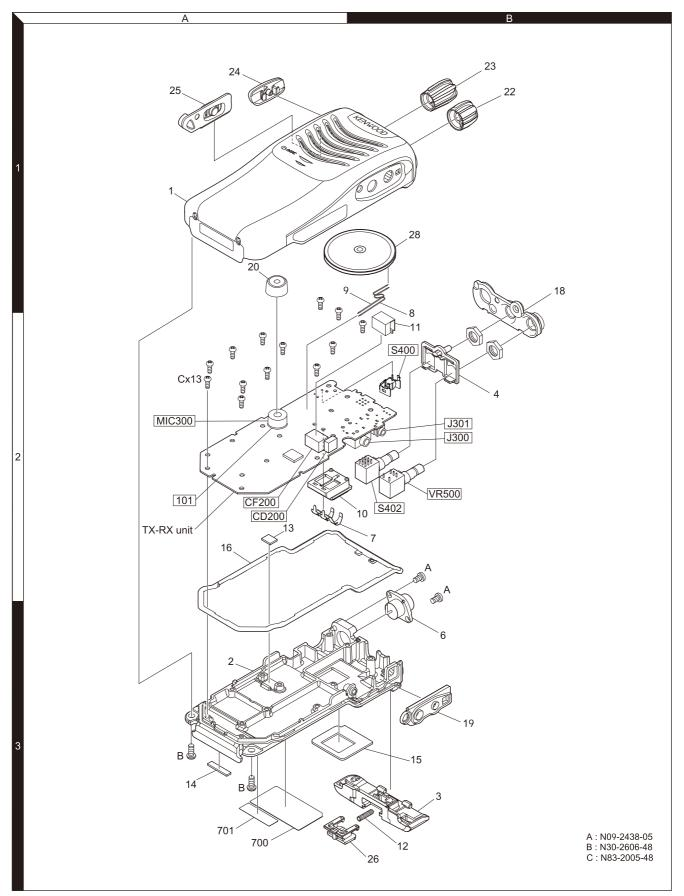
Parts with the exploded numbers larger than 700 are not supplied. If a part reference number is listed in a box on the exploded view of the PCB, that part does not come with the PCB. These parts must be ordered separately.
